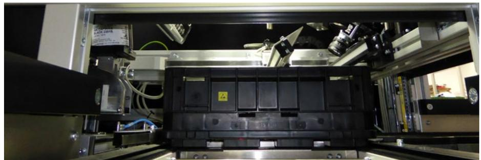
framework. The design of the machine had to take in account the loading and unloading by operators along with all the required tooling and fixtures for holding the vision system components and associated LED line lighting. The vision inspection area was purposely designed to stop the ingress of ambient light; therefore lighting levels could be controlled by automatic switching of the machine vision lighting arrays as
