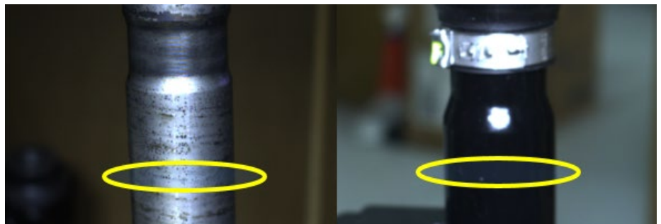
Figure 2: To check whether the correct size of drive shaft has been installed in each corner unit, an IVS monochrome camera captures an image of the shaft of the drive shaft which is backlit by a red LED unit. The image is then processed to determine the location of the edges of each side of the drive shaft from which its width, and the model of the drive shaft, then be determined.
