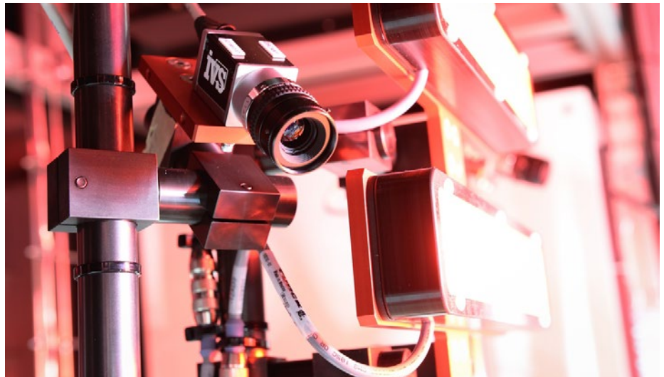
Figure 1a: An IVS CCD camera captures a monochrome image of the shaft of the drive shaft which is backlit by a red LED.
