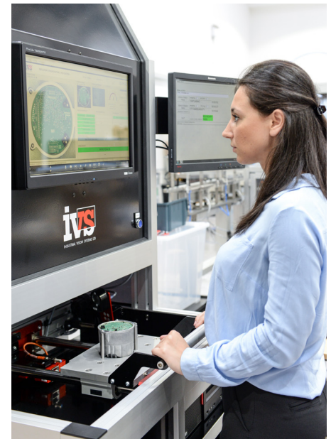
Figure 1: Industrial Vision Systems has developed a vision system for the inspection of a sealed electronic assembly. As a stand-alone unit, the system has been designed to check for correct PCB component placement, component defects, whether the unit is correctly housed and whether it has been correctly sealed.
