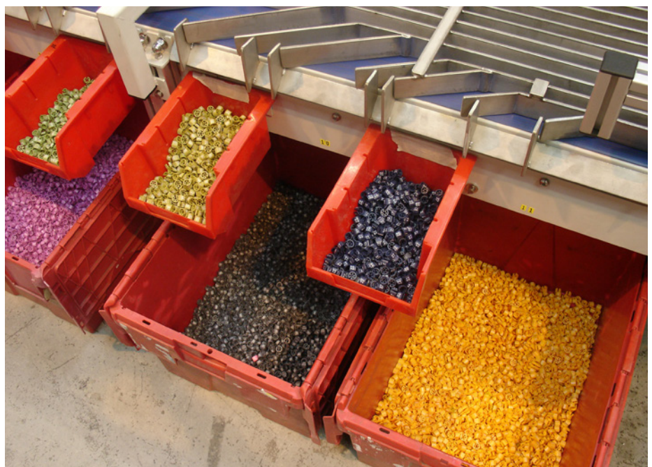
Actuators blow the cubes into their relative sorting bins
