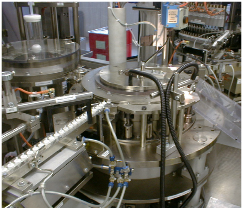
Rotary manufacturing table with vision system
