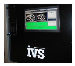
statistical process control for the products being manufactured for later analysis. Images of every product can also be saved and allocated against serial number tracking to allow photos of every product leaving the factory to be stored if required.
