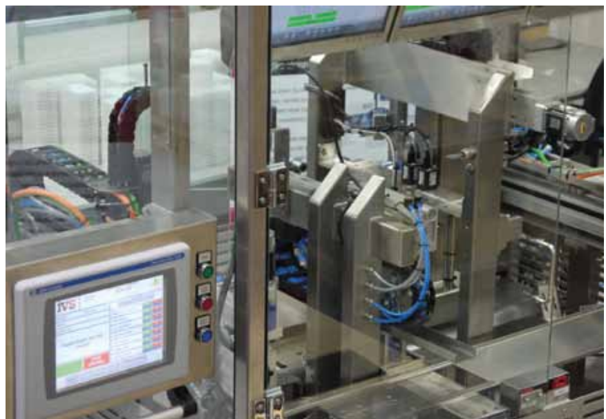
Figure 6: Having verified the color consistency of the wells and inspected them for contamination, the tray of wells is then indexed down the inspection line to a fourth station where any unacceptable wells are removed.
