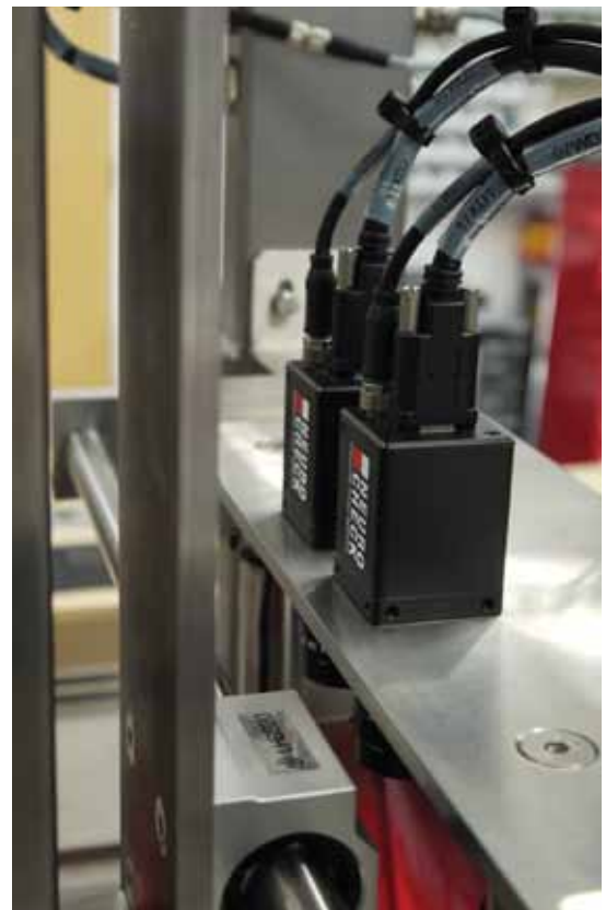
Figure 4: At the second vision inspection station, an image of the wells is captured by a pair of area scan cameras. Software then checks to determine whether the color of the wells meets specification and that there are no particulates inside the well.
