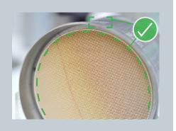
A highly flexible quality control inspection cell – CATi from Industrial Vision Systems lets you automate repetitive and critical inspection tasks on catalyst parts utilizing latest linescan sensor technology to leverage highly accurate quality control. CATi uses artificial intelligence vision sensors to provide mission critical quality inspection criteria across the entire production cycle.
